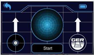
Turn in the opposite direction, press the start button, wait until you hear a beep emanating from the device, and the icon shifts from the rotation position to the forward position, then walk until the device rotates backwards, the device will analyze and show the final results automatically.
