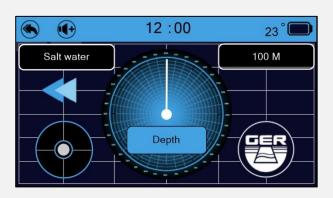
After you have confirmed the location of the target, click on the depth button to determine the depth and then move away from the center of the target a distance of at least two meters.
