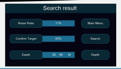
The following results and conditions will appear on the device screen when confirming the presence of a target:
