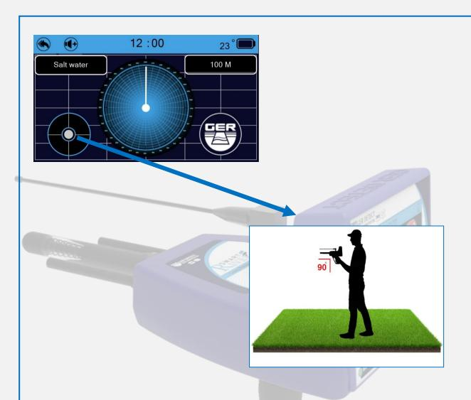
The balance of the device must be maintained during the search by fixing the grey dot in the middle of the circle icon.
