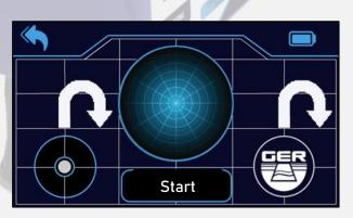
Point the device towards the target while maintaining the balance of the device, press the start button, wait until you hear a beep from the device, then walk towards the target until the device rotates backwards with the appearance of an icon indicating the rotation of the device towards the back.
