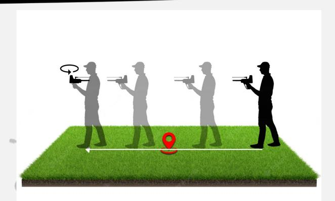
Follow the signal and when the device turns back you will have passed the target
