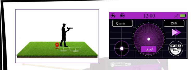
After you have confirmed the location of the target, click on the depth button to determine the depth and then move away from the center of the target a distance of at least two meters.
