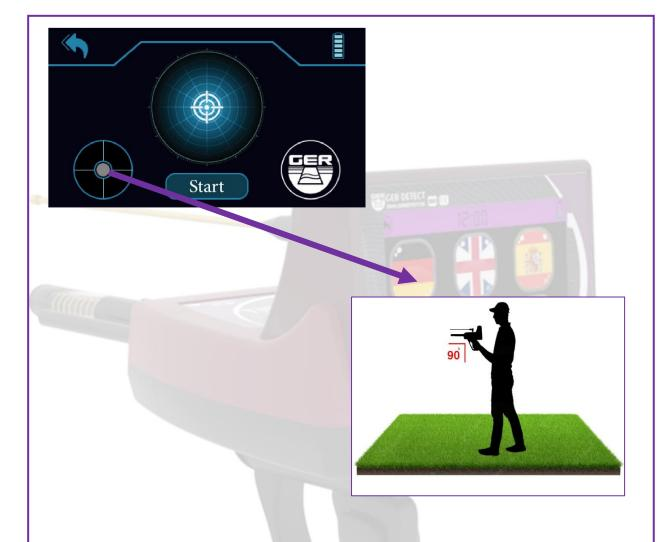
The balance of the device must be maintained during the search by fixing the yellow dot in the middle of the circle icon.
