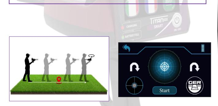
Point the device towards the target while maintaining the balance of the device, press the start button, wait until you hear a beep from the device, then walk towards the target until the device rotates backwards with the appearance of an icon indicating the rotation of the device towards the back.
