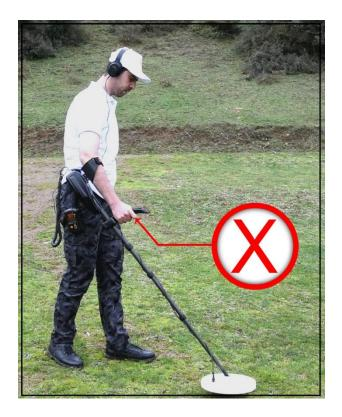
NOTE: Don't press the calibration button while working on the device.
