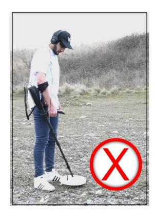
Avoid the continuous friction of the coil with the ground and rocks.
