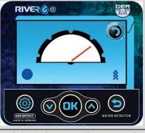
2- When the water source is on the left side of the device, the antennas and the indicator will move to the left direction and a beep sound will start accelerating, alerting the user to follow the water source.
