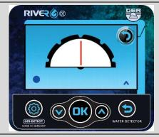
1- When the water source is on the right side of the device, the antennas and the indicator will move to the right direction and a beep sound will start Accelerates alerting the user to follow the water source.
